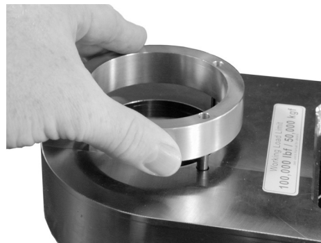
Figure 7.4 Placing Second Spacer on Roll Pins
