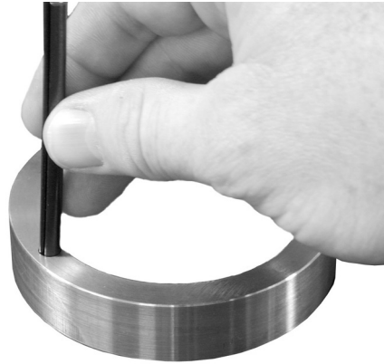
Figure 7.2 Inserting Roll Pin
